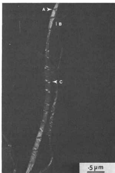
Figure 9. Electron micrograph showing orientation effects on the banded structure
